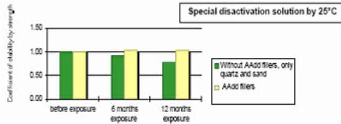
\*\*\*AAdd in non-burning monolithic flooring provides upgraded chemical resistance against special disactivation solutions. Materials with AAdd are able to pass the IAEC method test for "natural fire" burning where flooring materials without the additive cannot.
